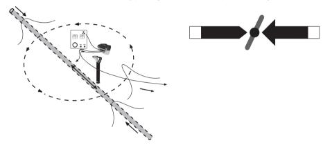
Keeping the receiver pointing at the connection point, walk around the connection point for a full 360 degrees. The reading on the receiver signal strength meter will rise and fall as it passes over:
