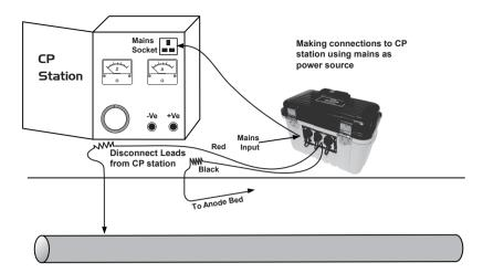
4. If there is no mains socket, it is possible to use the DC output of the transformer rectifier. See diagram below.
