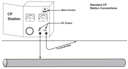
3. Disconnect the output wires connecting the CP station to the pipeline and anode bed. If there is an earthed mains socket at the station, connect the transmitter mains power lead to the socket.
