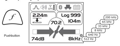
The receiver is capable of detecting a large number of frequencies. To simplify the operation of the equipment, it is possible to activate only frequently used frequencies. This is done by entering the user menu.
