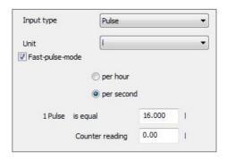
The checkbox Fast-pulse-mode must be activated if a sensor is used with a pulse rate >50 Hz (ie, more than 50 pulses per second). Otherwise, it may result in inaccurate measurements.
