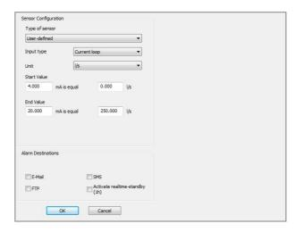
The sensors contained in the list are parameterized. The signal conversion data are already populated and cannot be edited. Usually, no further configuration is required.
