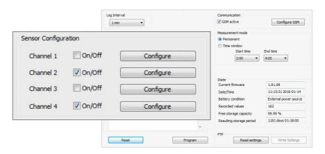
Configuring a channel After a channel has been activated, it has to be specified which type of sensor is connected to the channel.
