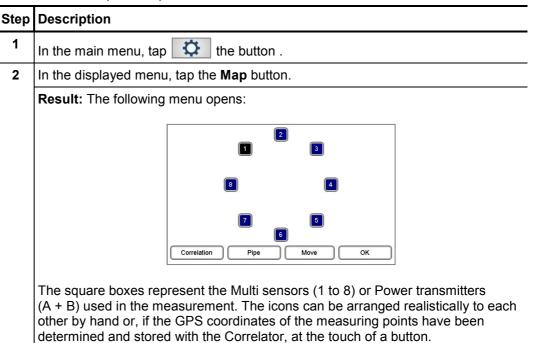
Arrange sensor icons The sensor icons can be moved and repositioned on the screen. (Only possible via touch screen, not possible via rotary encoder).
