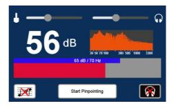
5 Adjust the **microphone gain** for the pinpoint location using the slider at the top left of the screen.
