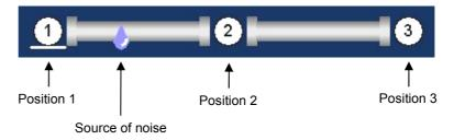
5 Select the sensor which represents Position 1 (sensor "in front of" the sound source) by tapping the required box.
