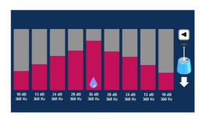
After the first After the first pinpointing run is performed, you know the approximate location of the pinpointing run leak. Furthermore you have an idea of the frequency spectrum and you are able to assess whether the microphone gain needs to be changed or not.
