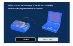
Connect the Correlator to the computer. Use the supplied connection cable. 5 (Connect the round plug of the cable to the **USB / GPS** socket of the Correlator. Observe the markings on the plug and socket. You must feel the plug engage.)
