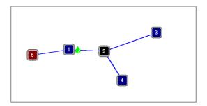
The correlation of the line from sensor 5 to 3 results in a leak at the very same position.
