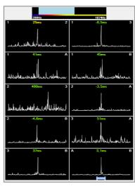
Set frequency filters The frequency diagram at the very top of the screen allows you to set a frequency filter and to repeat the correlation.
