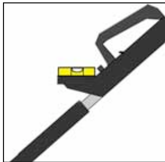
A bubble level on the meter panel will tell you when you are holding it at 45°
