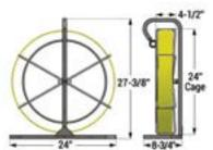
Minimum bend radius is 7" and sizes available are from 150' up to 500'. DCD does not recommend pushing lengths over 500' unless in relatively small ducting 2" dia. or smaller.
